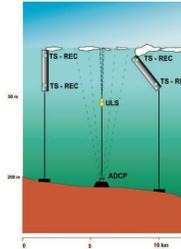
Scheme of tube mooring array (left). The approximately 40 m long tube protects the instruments against damage due to ice. An Upward Looking Sonar (ULS) was not used. There is a security line attached at the outside of the tube, in case of breaking. Positions of tube moorings and ADCP are shown below on the East Greenland Shelf, with water depths and depths of temperature and salinity.
